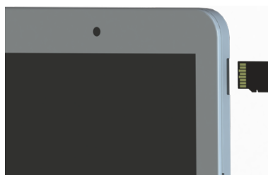
Figure 4. Inserting and Retrieving a Micro SD Card
